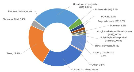
Table 3: Weight of materials XT6 IEC 3P 800 N/S/H Ekip Circuit Breaker
