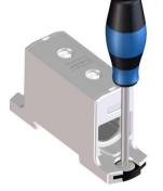
**DIN-rail mounting** Set the connector to DIN-rail. See picture. Push until "click"
